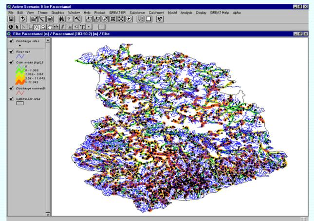
Fig.2 GREAT-ER user interface with result map for Paracetamol in the Elbe catchment
