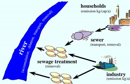
Fig.1 GREAT-ER chain of models and simulated processes
