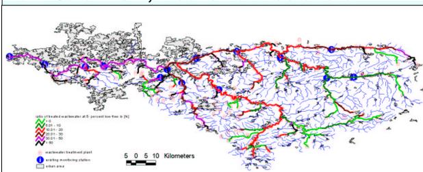
Fig. 7 Fraction of Urban Wastewater in Ruhr Catchment at 5 % Low-Flow
