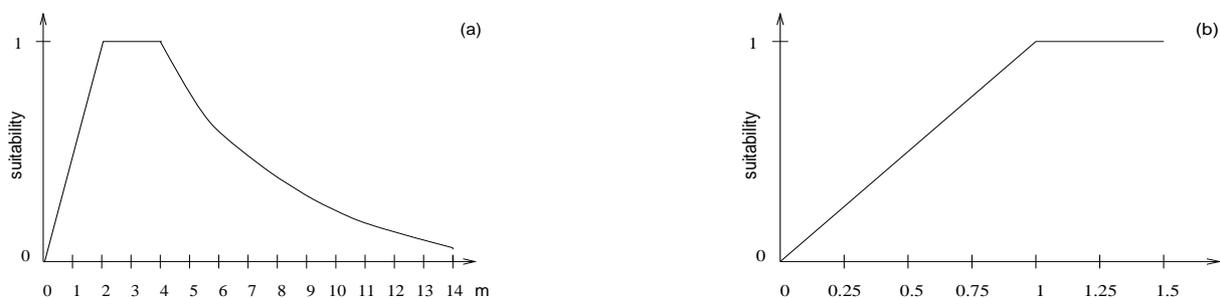
Figure 7.4: Suitability curves of (a) the ground water level and (b) the flooding frequency for adult *P. euphratica* individuals.
