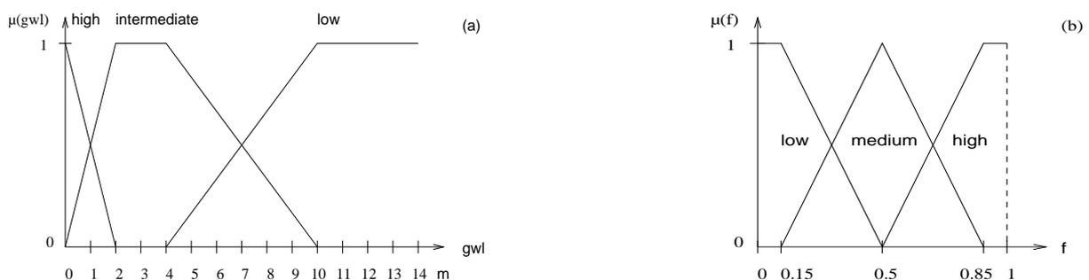
Figure 8.2: Fuzzification of (a) the ground water level (gwl) and (b) the suitability of the flooding regime (f).
