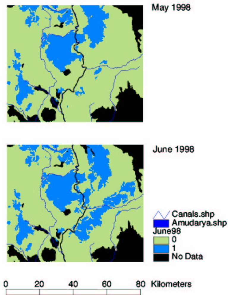
Figure 6.3: Flooded areas during the flood in May (above) and June 1998 (below). 0 - not flooded, 1 - flooded. Data provided by Schlüter.
