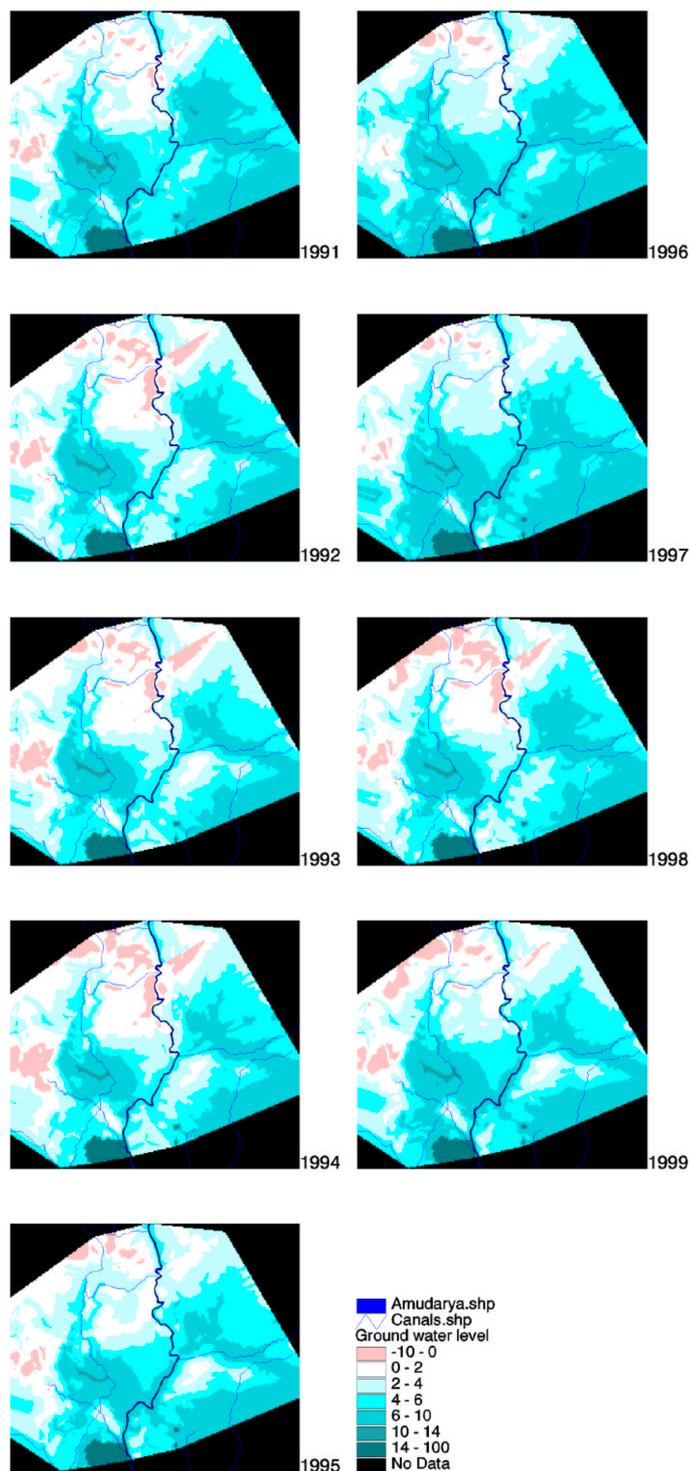
Figure 6.2: Development of the ground water level from 1991-1999. Data interpolated from measurements at 25 wells across the delta area and provided by Schlüter. For details about the interpolation see Schlüter (in prep.).
