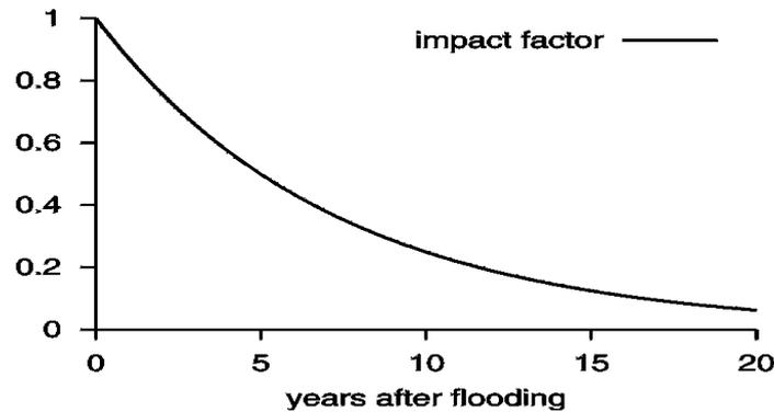
Figure 7.1: Exponential decay of the impact factor of a flooding.  $f(x) = e^{-0.14x}$ .
