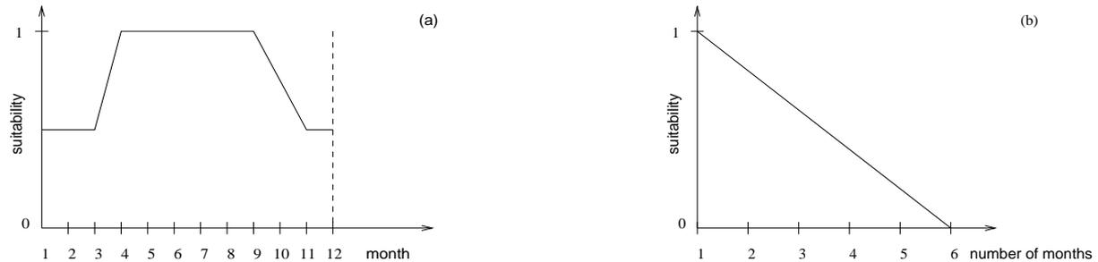
Figure 8.1: Suitability curves for the flooding timing (a) and the flooding duration (b) of an additional flooding.
