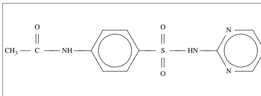
**Figure 3.1:** Chemical structure of  $N_4$ -acetyl-sulfadiazine
